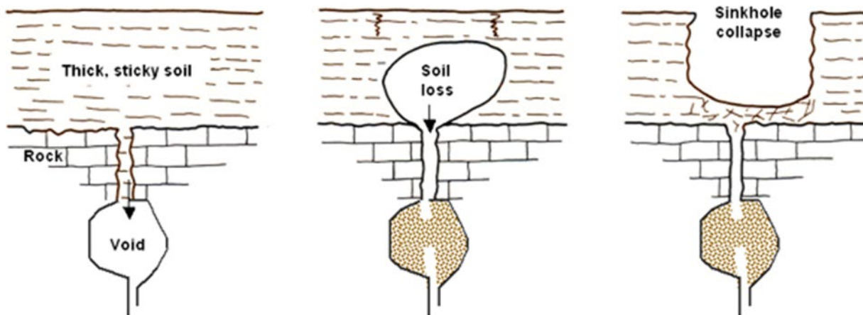
Figure 4.9.3 Sinkhole Formation Illustration
